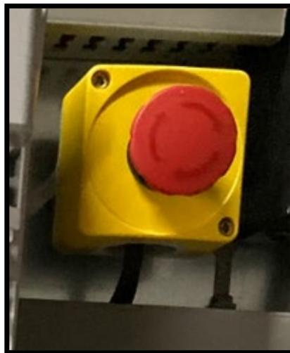
Fig B. Coupure AU
